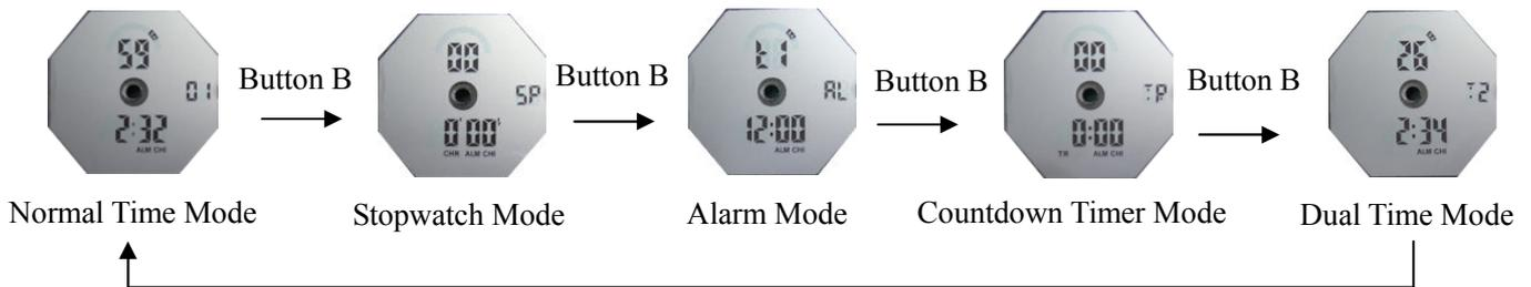
**1. In any mode, EL illuminates for 3 seconds by pressing A button. In non-setting mode, press B button to select operating mode.**
