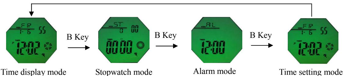
**1. Under any mode, press and hold A key to lighten EL for 3 seconds, press B key to select operation mode.**
