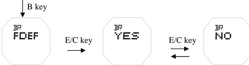
Factory default air pressure mode during the factory default air pressure setting
