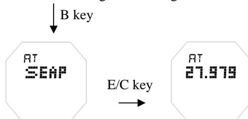
Input sea level air pressure      during sea level air pressure inputting
