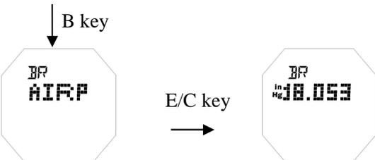
Input the current air pressure value during current air pressure value inputting
