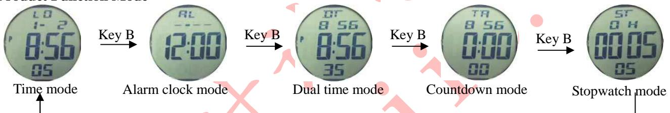
**1. In any mode, press key A that EL will light for 3 seconds, press key B to select operating mode.**
