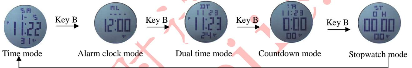
1. In any mode, press key A that EL will light for 3 seconds, press key B to select operating mode.
